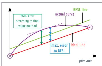
Non-linearity is also shown as BFSL (Best Fit Straight Line) as a reference value in the technical specifications. Non-linearity generally has the biggest influence on the overall error rate. Typically, non-linearity as per BFSL corresponds to half of non-linearity as per the full scale method ( $1\% \text{ FS} \sim 0.5\% \text{ BFSL}$ ).
